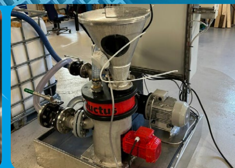
The water lock and pump system in one compact unit
